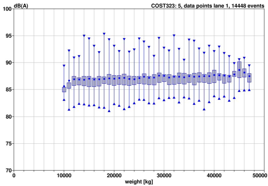
Figure 7.9: Maximum pass-by levels [dB(A)] for COST 5 vehicles in different weight classes.
